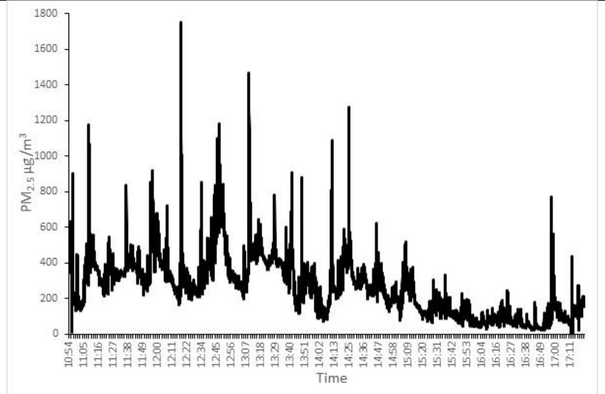
Data are values from a factory-calibrated laser photometer, corrected for biomass smoke. (Dustrak model 8532, TSI Inc, Shoreview, MN)
